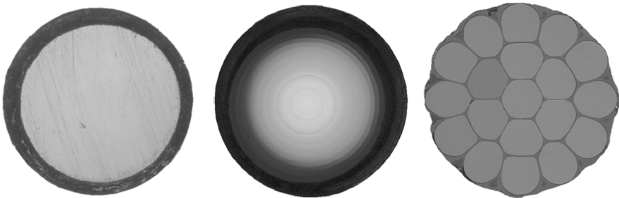
Fig. 2: Step index-, multi step index- and multi core polymer fibers
